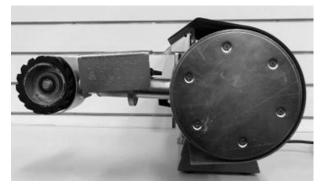
Install the guard (F) over the assembly and tighten the 3 x cap screw (G).
