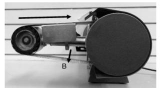
Push against the contact wheel towards the drive pulley to retract the extension arm and place the linishing belt (B) over the main wheel and the contact wheel. Refer to the inside of the belt for the correct installation direction of the belt.
